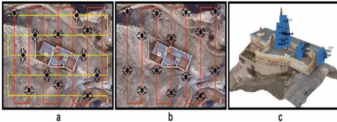
**Figure 4.** Flight plans; a) multi-orientation, b) 2D photogrammetry and c) manual photography
