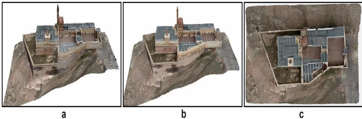
**Figure 5.** Ishak Pasha Palace photogrammetric adjustment process results; a) point cloud, b) 3D model and c) orthophoto
