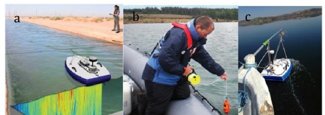
Figure 5. ADPD – a) device conceptual view; b) CastAway CDT device usage [47]; c) device usage on site
