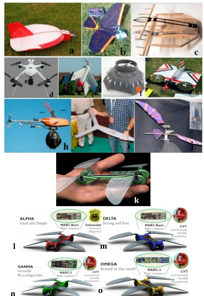
Figure 4. Different types of MAVs, (a) fixed wing, (b) flapping wing, (c) fixed/flapping-wing, (d) rotary wing, (e) VTOL, (f) ducted fan, (g) tilt-rotor, (h) helicopter, (i) unconventional, (j) ornithopter [11], (k) TechJect Dragonfly fits in the palm of a hand, (l) Alpha model Dragonfly, (m) Delta model Dragonfly, (n) Gamma model Dragonfly, (o) Omega model Dragonfly [53]
