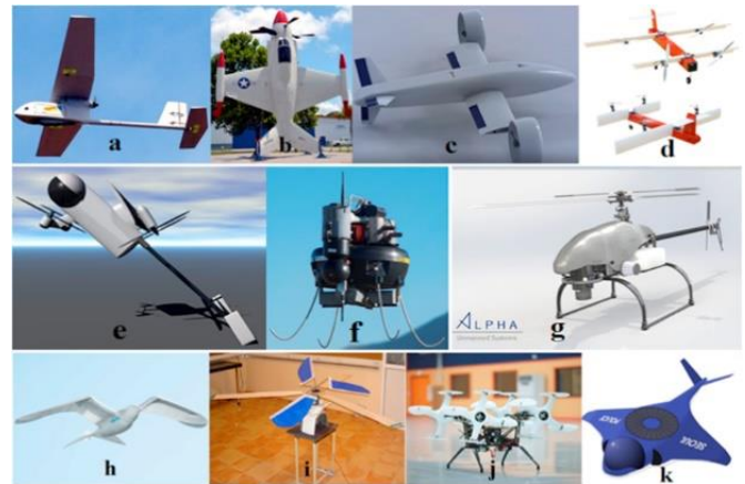
Figure 3. Different types of \mu UAVs, (a) HTOL, (b) VTOL, (c) tilt-rotor, (d) tilt-wing, (e) tilt-body, (f) ducted fan \mu UAV, (g) helicopter, (h) ornithopter, (i) ornicopter, (j) cyclocopter, and (k) unconventional \mu UAV [11, 36, 37]
