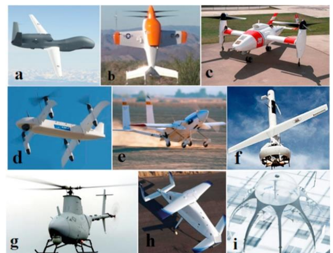
Figure 2. Different types of UAVs, (a) HTOL, (b) VTOL, (c) tilt-rotor UAV, (d) tilt-wing UAV, (e) tilt-body UAV, (f) ducted fan UAV, (g) helicopter, (h) heli-wing, and (i) unconventional UAV [11, 26, 27]
