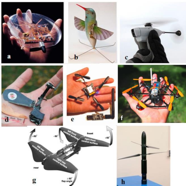
Figure 5. Different types of NAVs, (a) fixed wing [62], (b) flapping wing [63], (c) helicopter [64], (d) monocopter, (e) quadrotor, (f) hexacopter, and (g and h) unconventional [11]
