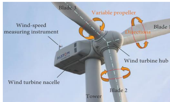
Figure 3. The implementation of pitch angle [41].
