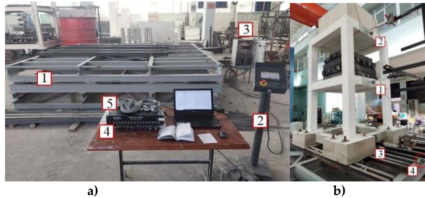
Figure 7. a) Experimental setup; 1) shake table, 2) control panel, 3) PLC-controlled automation system, 4) data acquisition system, 5) accelerometers, b) Sensor locations; 1) 1. story sensors, 2) 2. story sensors, 3) potentiometer on the foundation, 4) accelerometer on the shake table platform
