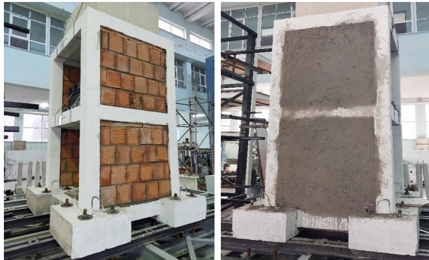
Figure 12. Improvement with infill walls
