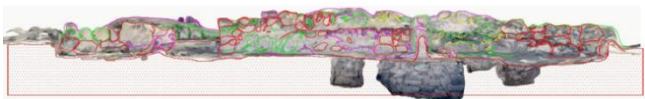
Figure 22. Section drawn in autocad environment over the orthophoto taken with Polycam programme.
