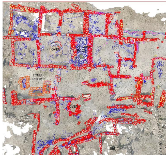
Figure 15. Plan drawing drawn on orthophoto created with Agisoft metashape programme.
