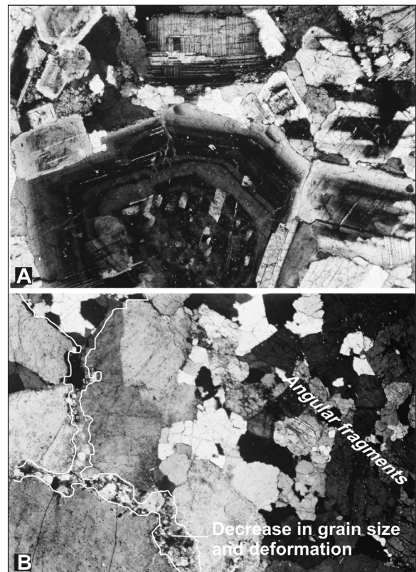
Figure 3- Photomicrographs of samples: a zoned crystal in granodiorite at inner parts of the pluton (A) and intense cataclasis along N-S trending contact zone (B).
