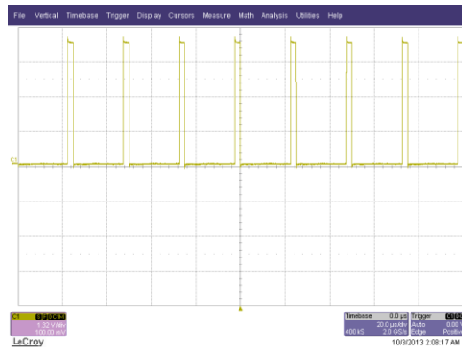
(b) Switching signal at 5% duty cycle
