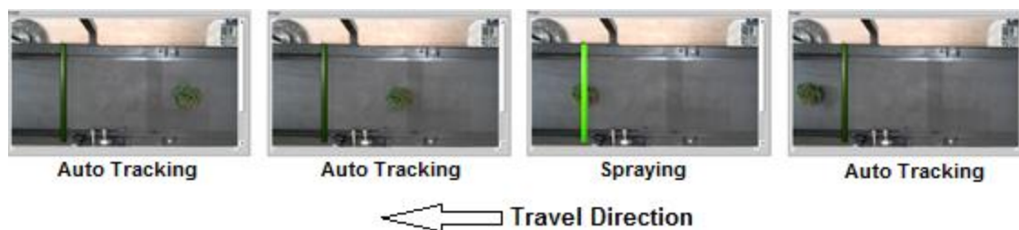
Figure 3. Real-time auto tracking and spraying of artificial weed sample in the laboratory
