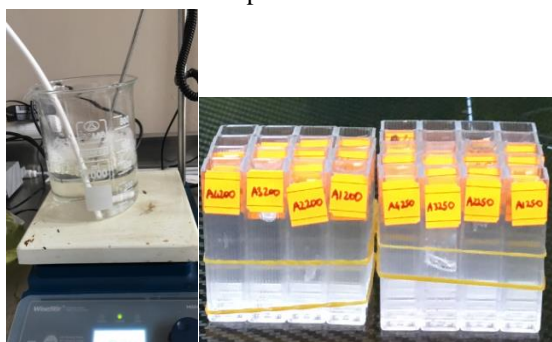
Figure 1. Gel samples in cuvettes and preparation of them.
