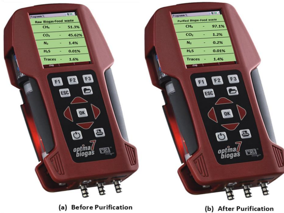
Figure 3. Optima Biogas 7 for determination of biogas composition
