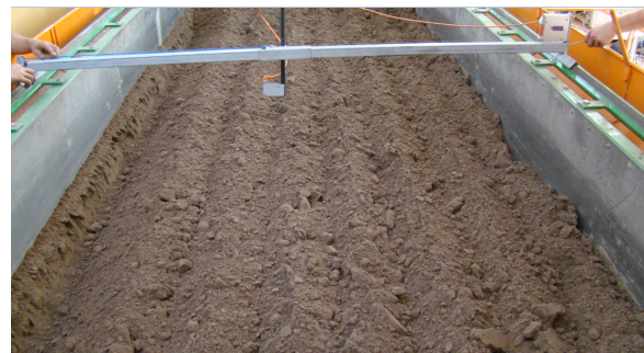
Figure 6. Soil profile measurements by laser in the soil bin
