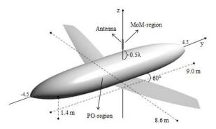
Figure 6. MoM and PO-region distribution for aerial vehicle example
