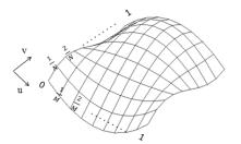
Figure 2. Mosaic of integration cells on the structure
