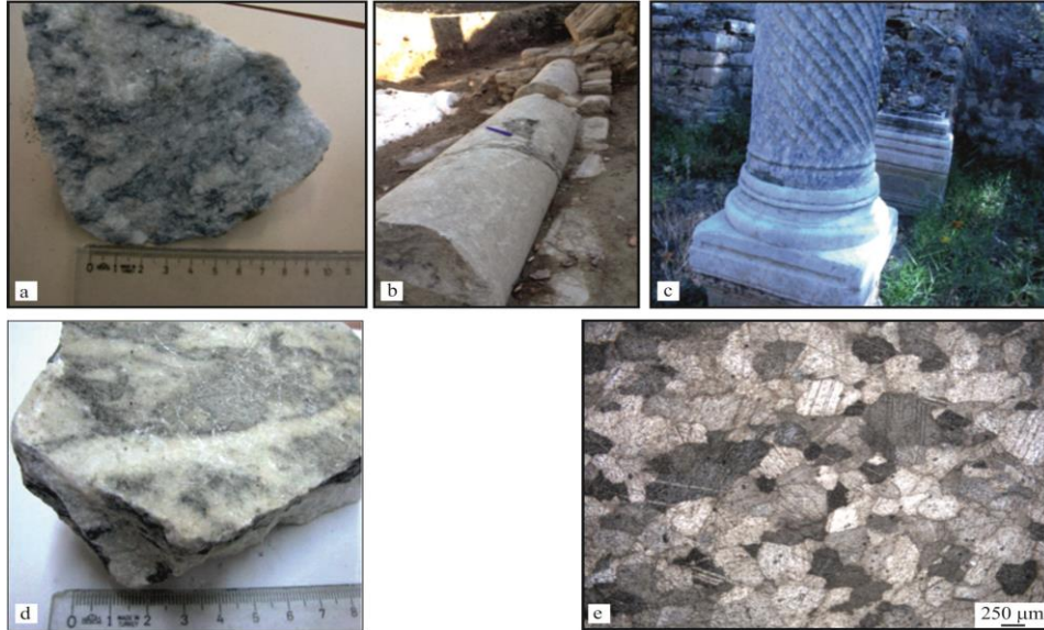
Figure 8. White gray marble used in monumental grave (a) and the same marble column in Aphrodisias (b-c). Macroscopic (d) and microscopic (e) view white-gray marble with medium crystal (thin section/2x-Cross polar
