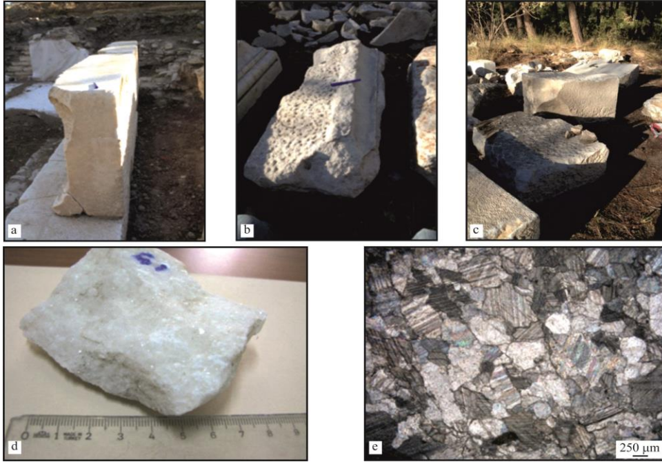
Figure 7. White marble type used in monumental tomb construction (a, b, c) Macroscopic (d) and microscopic (e) appearance of white marble with medium crystal (thin section/2x-Cross polar)
