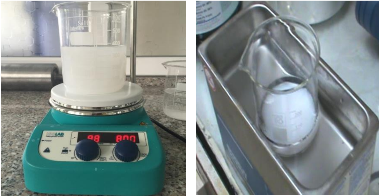
Figure 2. Nano-fluid ( BaTiO_3 -Ethanol).
