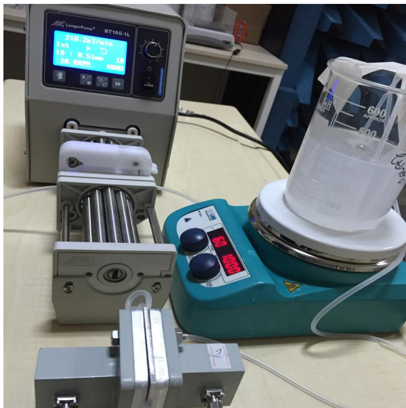
Figure 5. Nano–fluid pumping mechanism
