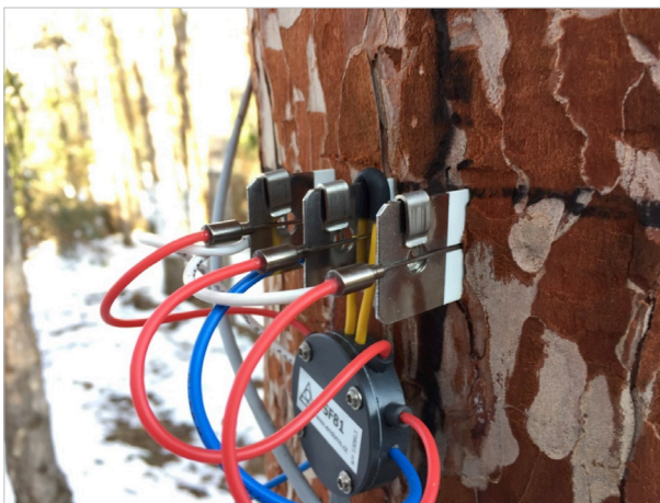
Figure 2. Electrodes, needle type thermocouples, isolator band and electric supplier hooks on the tree trunk
