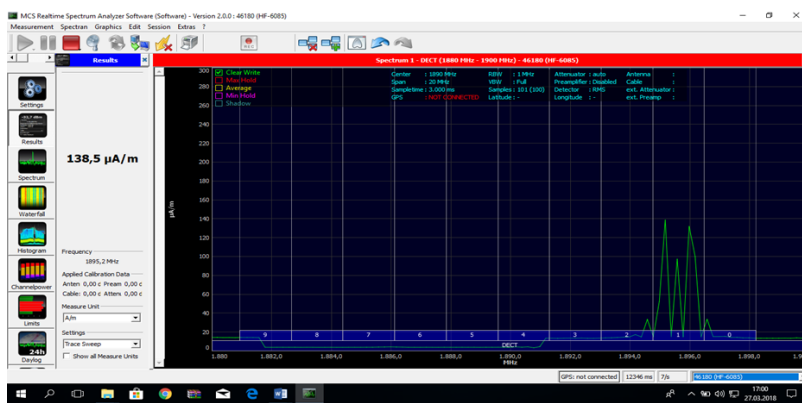
Figure 14. Magnetic Field Value for 30 cm Distance
