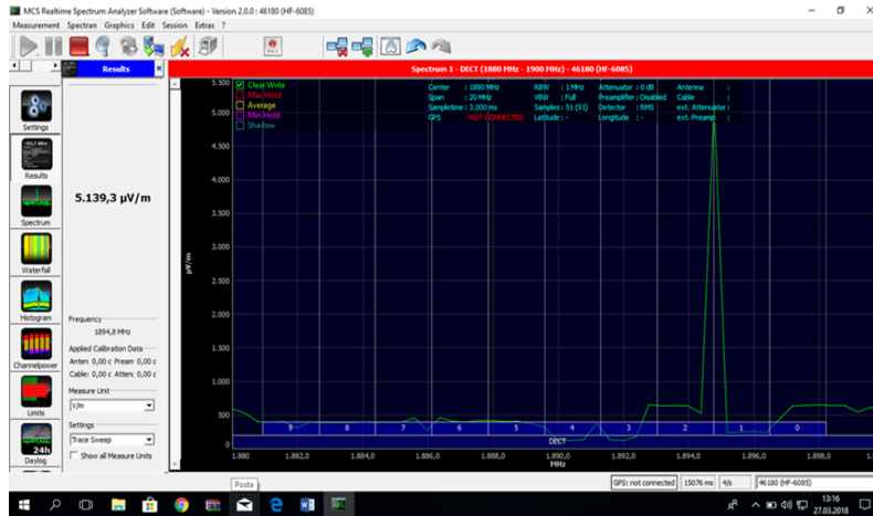
Figure 5. Electric Field Value for 1 cm Distance
