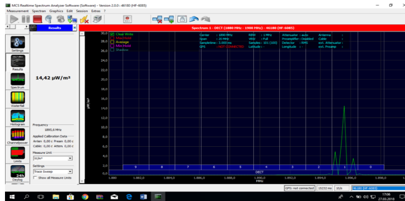
Figure 15. Equivalent Plane Wave Power Density (S) Value for 1 cm Distance
