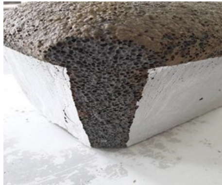
Figure 3: Standard (colorless) gas ceramic tile with foam structure.
