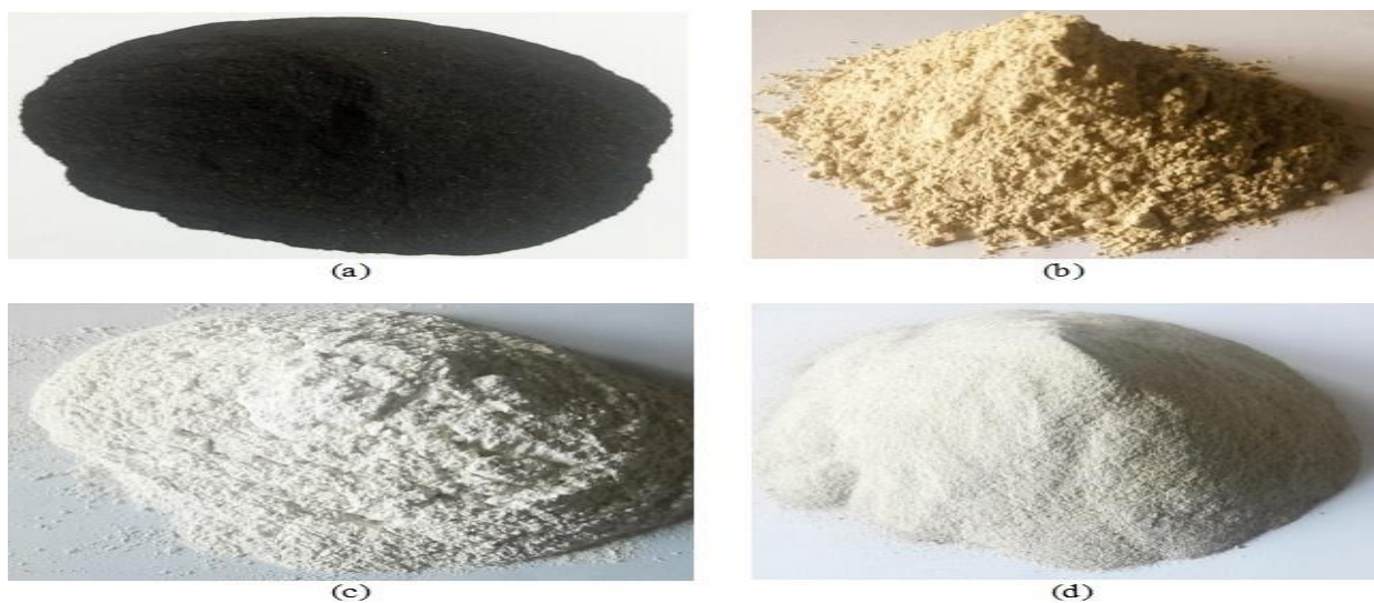
Figure 1. Photographs of input materials (a) 105 µm iron millscale particles, (b) 53 µm bentonite clay particles, (c) 80 µm magnesia particles, (d) 50 µm silica sand particles.
