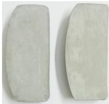
Figure 2c. Photograph of two samples of composite brake pads produced.
