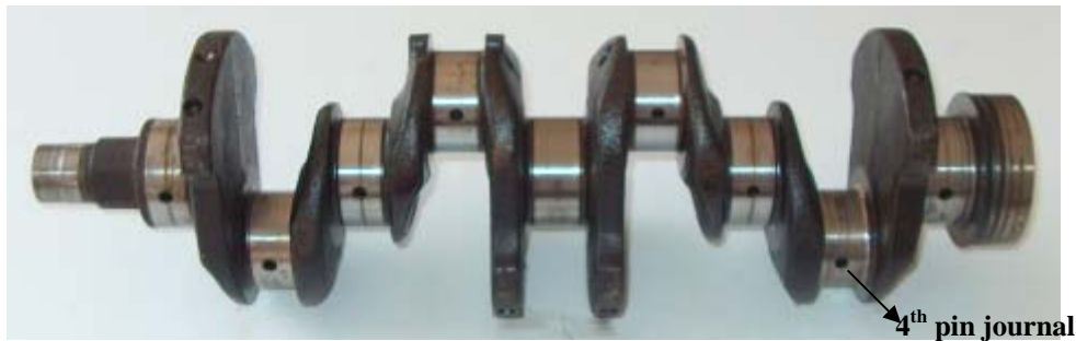
Figure 1. General appearance of the failed crankshaft
