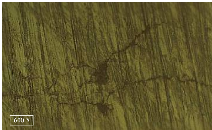
Figure 6. Formation of branch of a micro-crack
