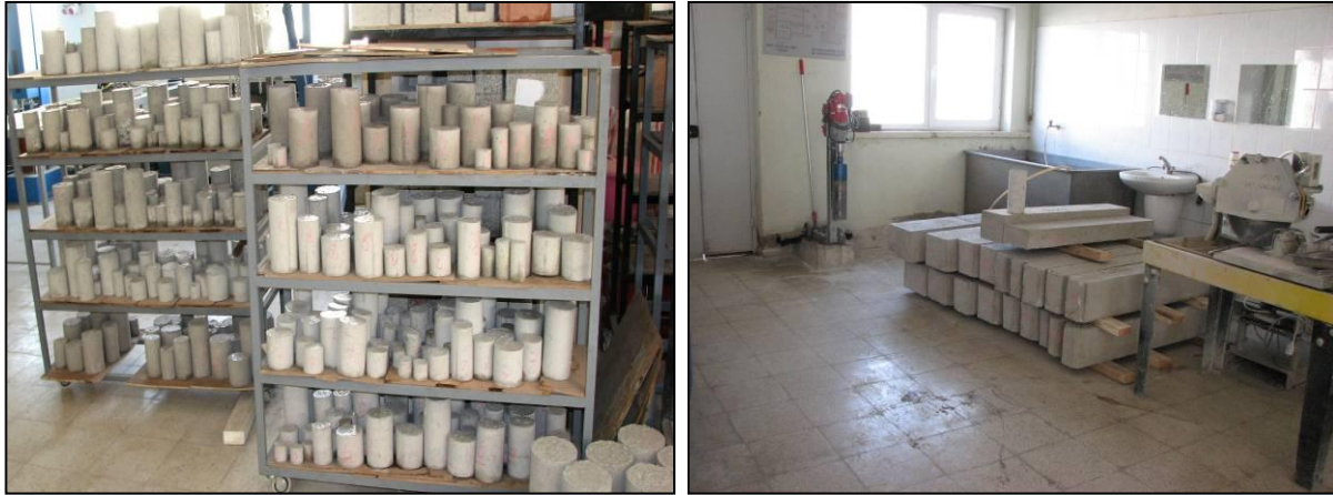
Fig.3. Reference specimens and blocks that would be drilled core for any series
