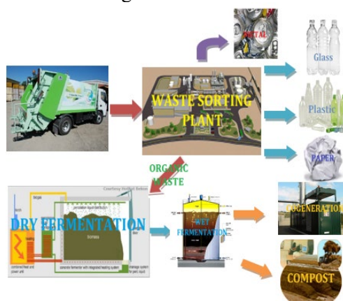
Figure 1. Solid / domestic waste recovery, recycling and flow chart of the power plant.
