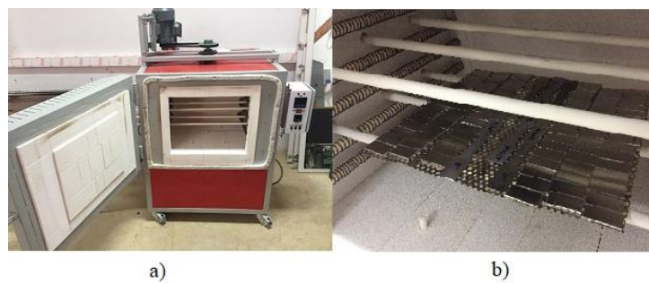
Figure 3. Annealing Environment (a) PID Unit Furnace; (b) Experimental Specimens.
