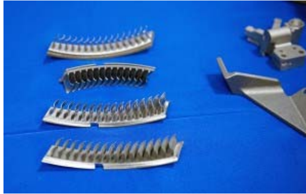
Figure 7. Image of Pratt Whitney jet engine that is produced with additive manufacturing with stator to be used in bombardier (Pratt-Whitney, 2015).
