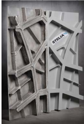
Figure 8. Trunk panel that is produced with additive manufacturing (Stelia, 2018).
