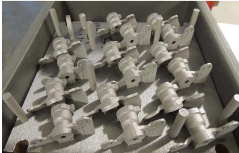
Figure 5. Image of 16 pieces of borescope eye and pulling samples being produced (Bamberg vd., 2015)
