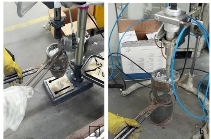
Figure 2. (a) Mechanical stirring, (b) ultrasonic vibration
