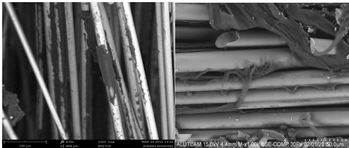
Figure 14. SEM images of produced plate samples-PP/E-glass composite structure
