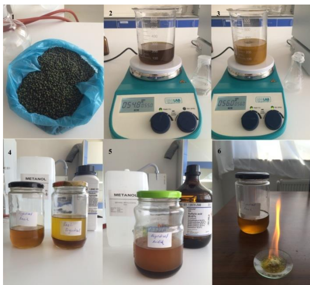
Figure 1. 1. Wild terebinth seeds, 2. Terebinth oil (dark green) heated at 55 °C, 3. Terebinth oil + methanol + NaOH solution in magnetic stirrer and heater, 4. Alkaline biodiesel with two phases: Biodiesel and Glycerol phases, 5. Acidic biodiesel with two phases: Biodiesel and Glycerol phases, 6. Deflagration of alkaline biodiesel
