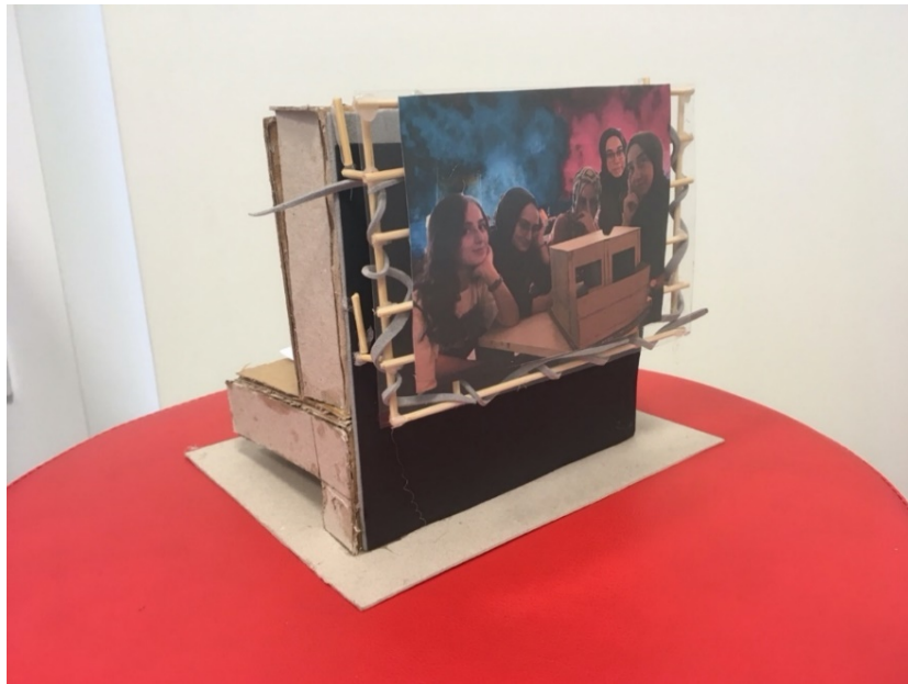
Figure 2. 1/10 scaled detail mockup – led screen wall surface
