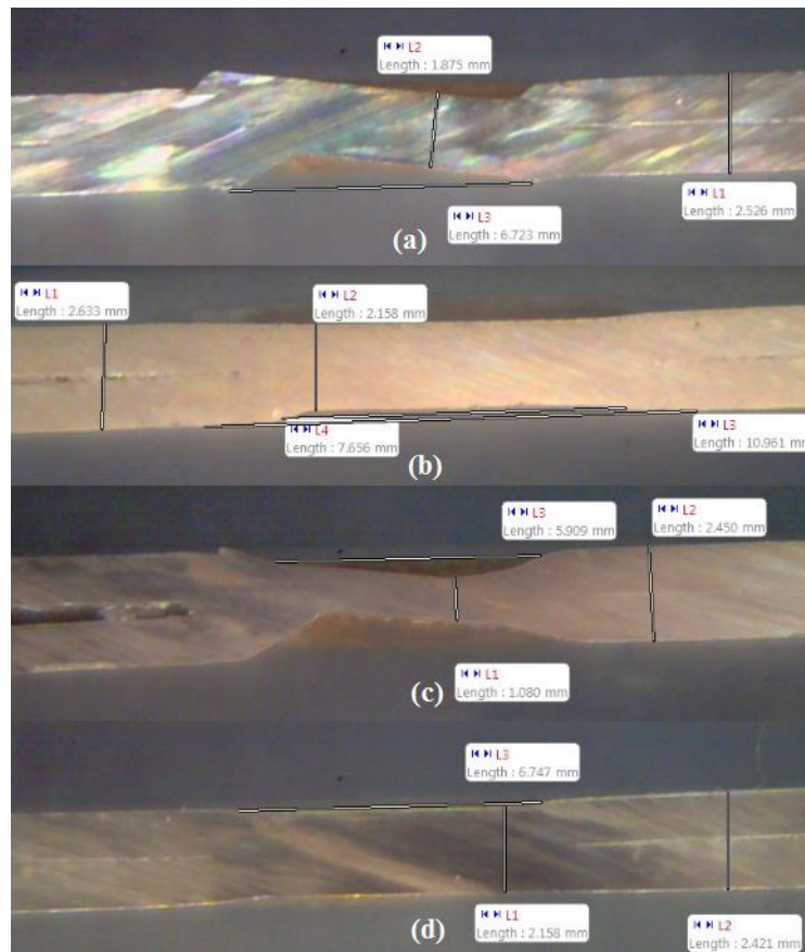
Figure 6. Macrostructures obtained at different electrode tip types at 5 kA welding current a) flat conical b) conical R3 c) conical round d) flat R6
