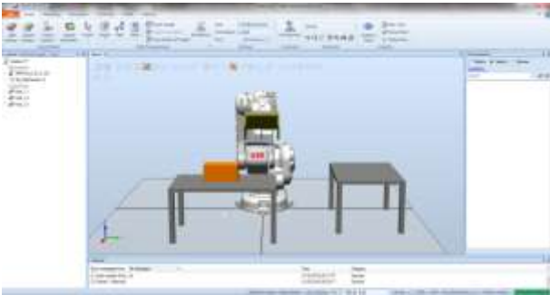
Figure 3. Designing the tables and the work piece
