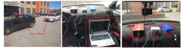
Fig. 2. Measurement setup: a) The transmitter and the receiver vehicle b) Inside of the transmitter vehicle c) Inverter, lighter splitter, DSRC OBU and camera.
