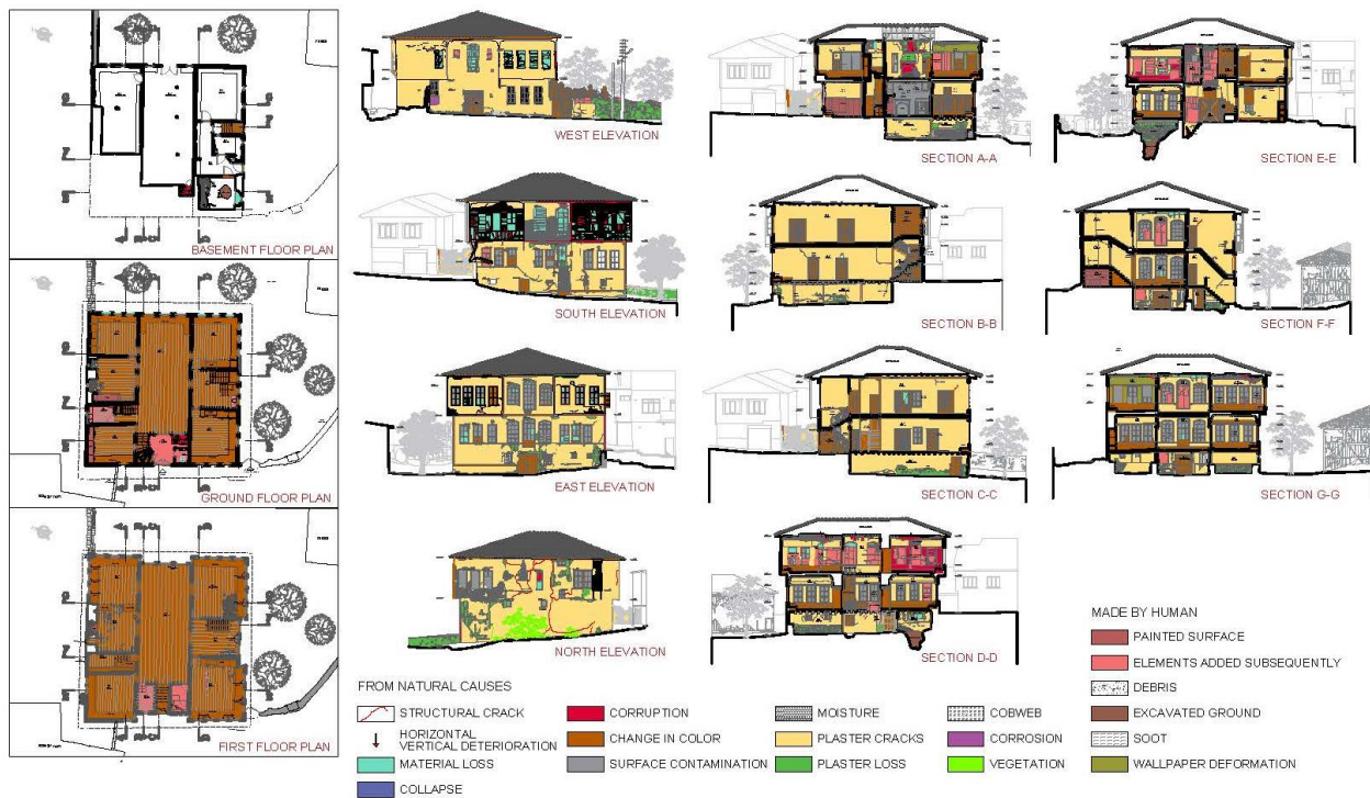
Figure 7. Deteriorations and corruptions
