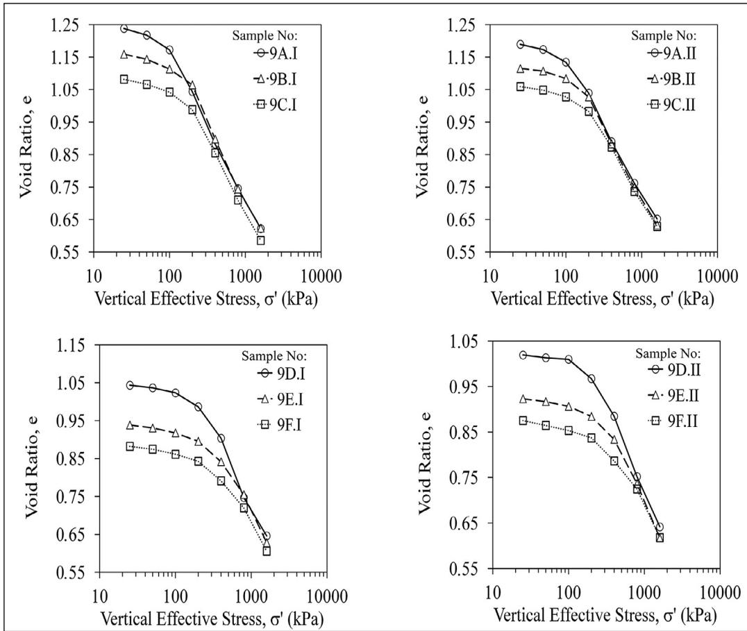
Figure 2-  $e-\sigma'$  curves obtained from conventional oedometer tests.
