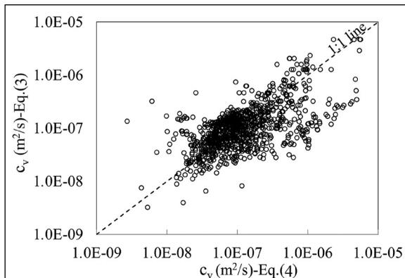
Figure 10- The comparison between  $c_v$  values calculated from Equation 3 and 4.
