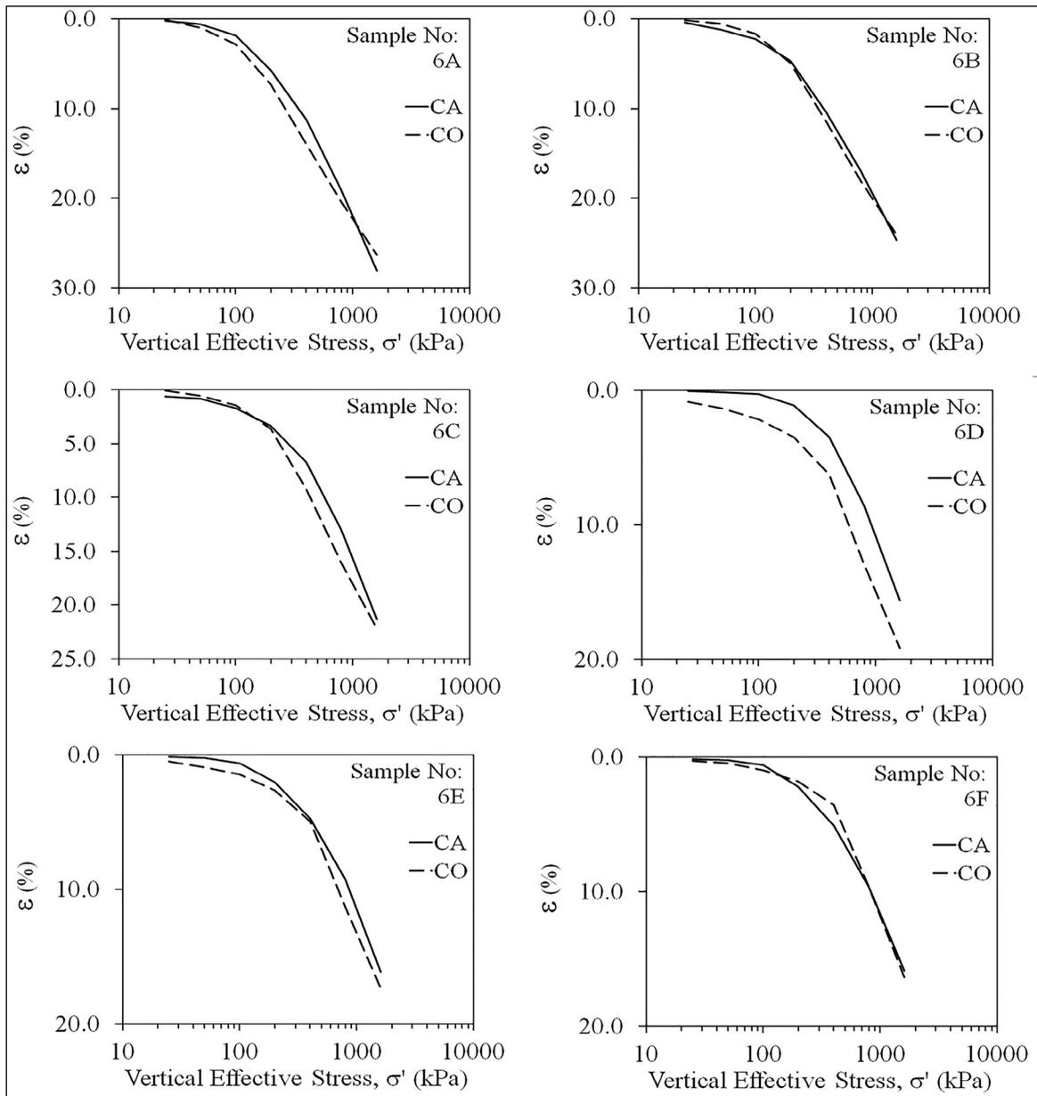
Figure 3- Comparison of the  $\epsilon$ - $\sigma'$  curves obtained from the conventional apparatus and the combined apparatus (CA: combined apparatus, CO: conventional 1D oedometer).
