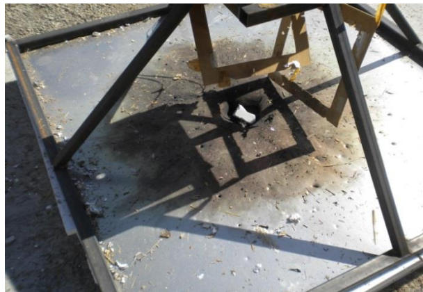
Fig. 5 Spall effect on the witness plate
