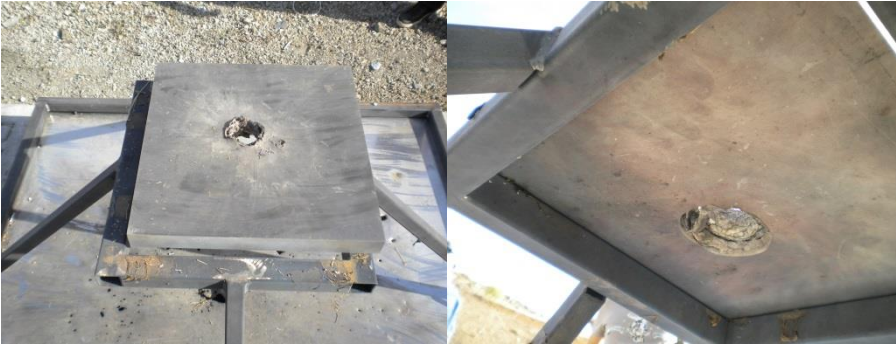
Fig. 6 Deformation of the Al5083 armor plate
