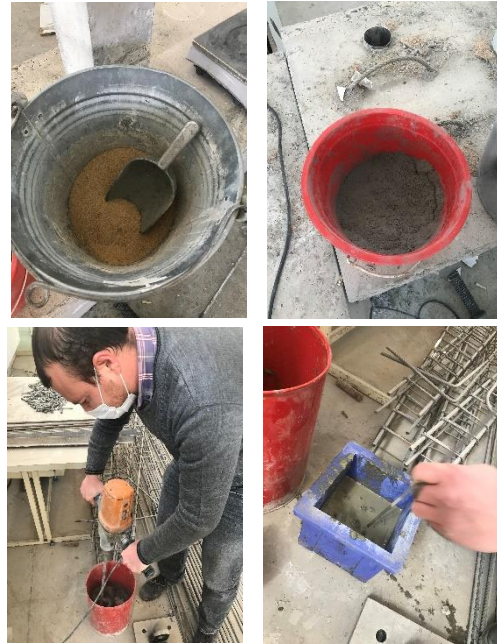
Figure 2. The concrete production process
