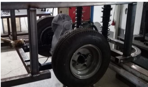
Fig. 21. Suspension and wheel system installation
