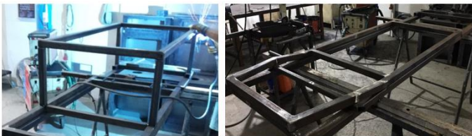
Fig. 20. a) Chassis manufacturing b) Welded chassis
