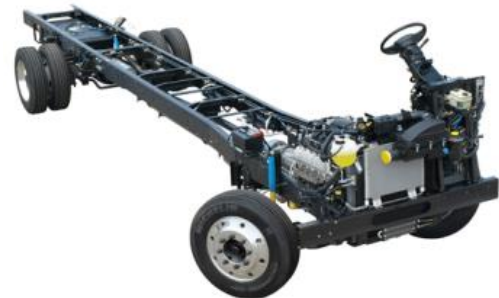
Fig. 3. Ladder type chassis [35]
