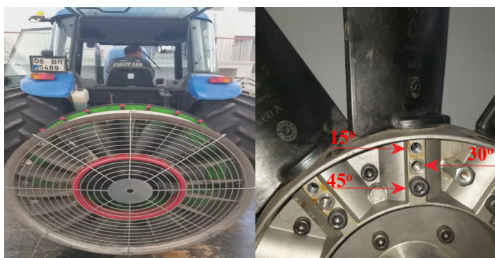
Figure 2. (a) The axial fan of the orchard sprayer and (b) aluminum fan hub blade angle change unit.
