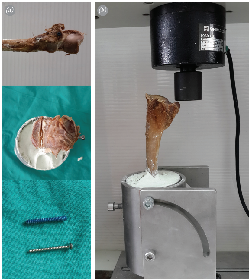
Fig. 1. (a) Screws tested. (b) Test set-up. [Color figures can be viewed in the online issue, which is available at www.aott.org.tr ]
