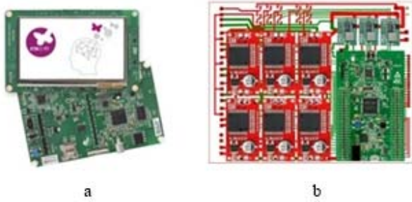
Şekil 10. Dokunmatik panel (a) ve koltuk kontrol ünitesi (b) (Touch panel (a) and seat control unit (b))
