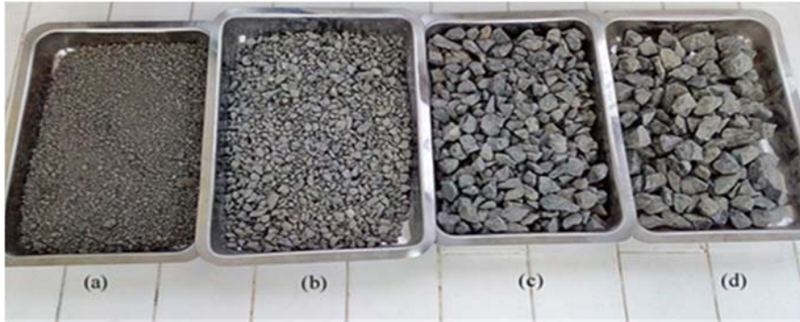
Şekil 2. (a) kırmataş tozu (0-5 mm), (b) micır 1 (5-12 mm), (c) micır 2 (12-19 mm), (d) micır 3 (19-37,5 mm) (a) crushed stone dust (0-5 mm), (b) crushed stone 1 (5-12 mm), (c) crushed stone 2 (12-19 mm), (d) crushed stone 3 (19-37.5 mm))
