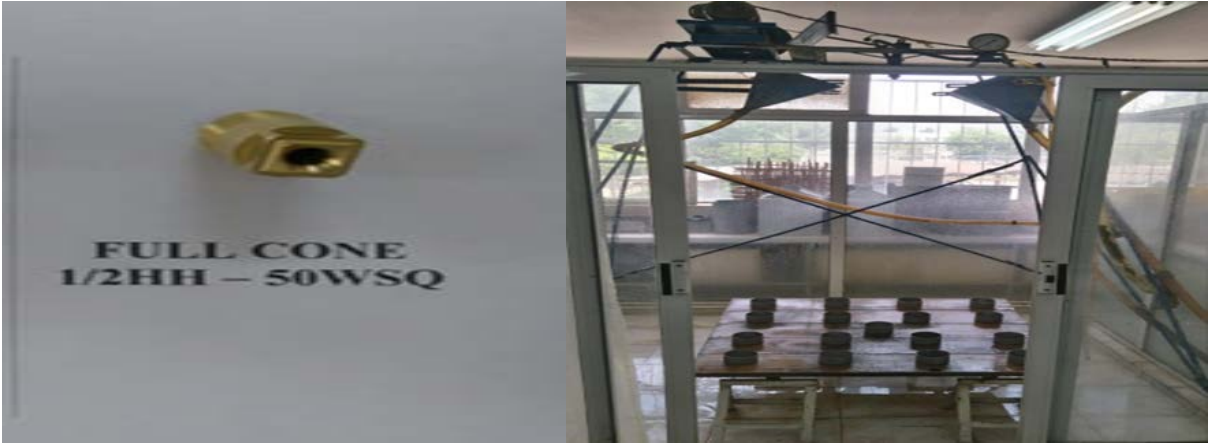
Figure 1. Full Jet type (1/2 HH-50WSQ) spraying nozzle, laboratory type rainfall simulator and cups of used in experiment.
