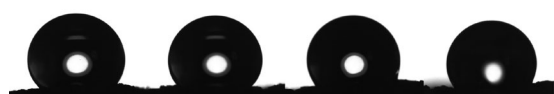
Figure 8. Sample images of water droplet CA measurements for the CSA-pumice sample (2 STs) from 141° to 117°.
