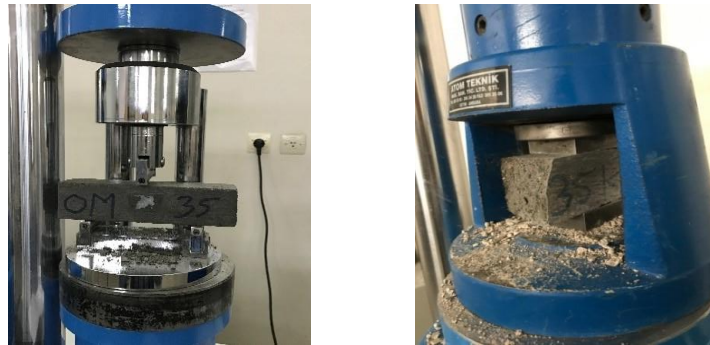
Figure 1. 3-point flexural (a) and compression test (b) of specimens
