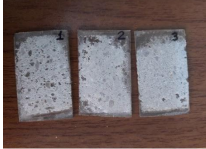
Figure 2. Thin sections extracted from specimens for petrographical analysis
