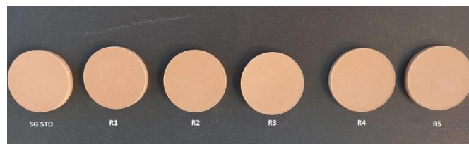
Figure 1 Fired porcelain tile tablets at 1185°C
