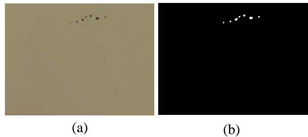
Figure 9 (a) Original CT image (b) defective binary image
