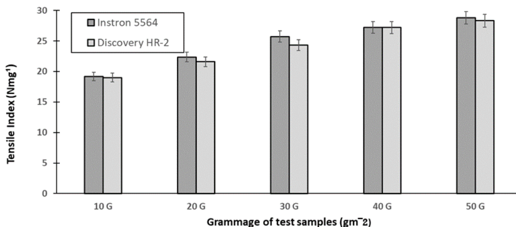
Figure 6 Comparison of tensile index values of paper groups obtained from two measurement ways
