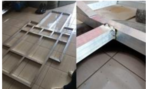
Figure 1: Chassis miter and welding work
