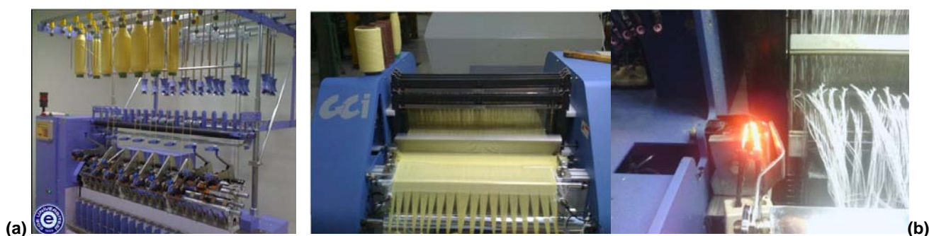
Figure 2. (a) Pinter – Merlin lab ring frame, (b) CCI SL 8900s weaving loom with new weft cutting system
