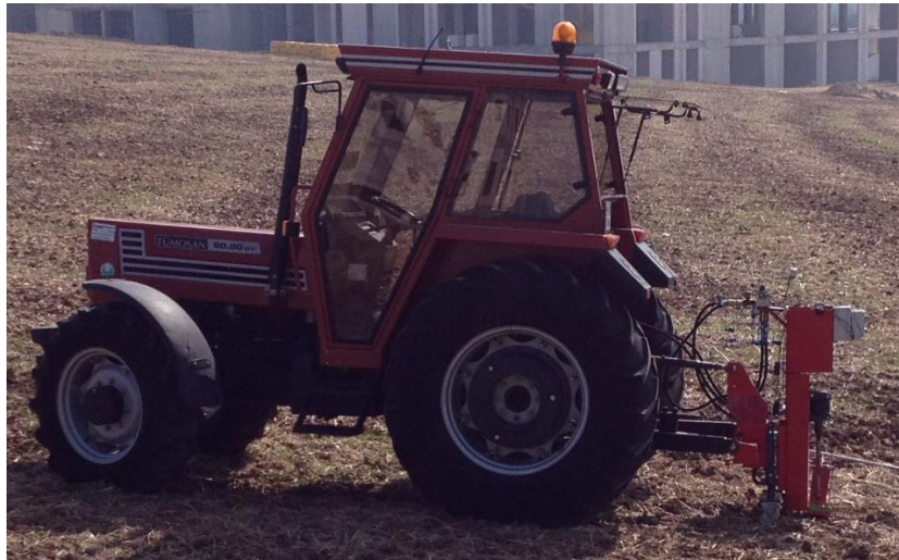
Figure 7. Soil sampling machine in field tests
