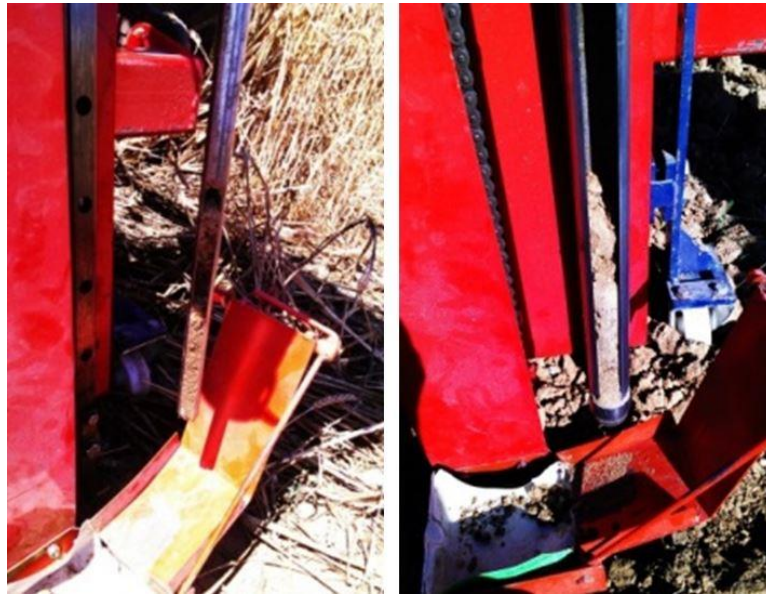
Figure 10. The soil samples on the type Ø12 and type Ø24 probes
