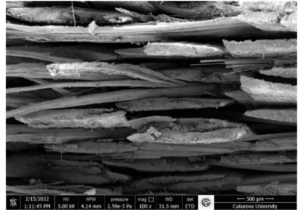
Figure 15. CE composites SEM micrograph
